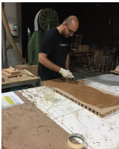
Applying glass fibers with resin
