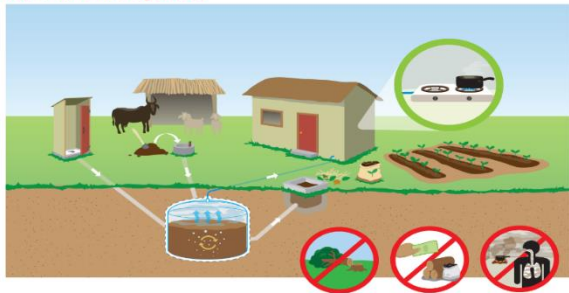
The Bio-Gas Digester:
